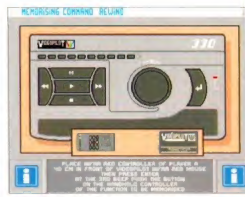
Like Gold Disk's Video Director, VideoPilot enables you to 'teach' its infra-red controller how to control your video deck.
